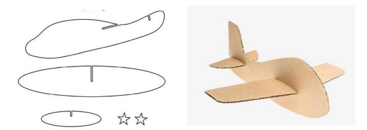
e.g of a cut and slot template, and a cardboard model
